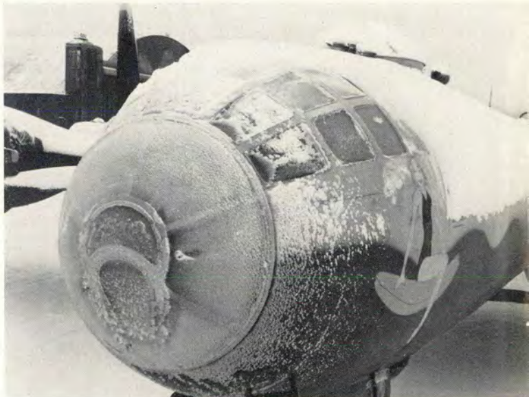
This B-29 nose shows ice picked up in flight
