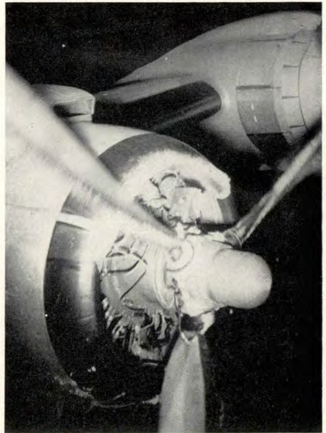
This photo shows ice forming on a propeller and engine of a C-54 which was used to fly missions in the USAF's research program on icing. Jet engines pose new research problems.
